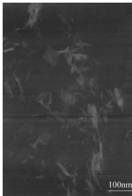
Figure 5 TEM micrograph of PBZ-PBO/OMMT nanocomposite (clay content 3%).
